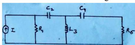
3. Find the current through  $5\Omega$  resistor by using superposition theorem.
