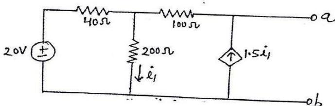
6. Find Thevenin's equivalent circuit for network shown in figure at the left of terminals n-y.
