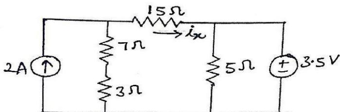
5. Find the Thevenin's equivalent of the network shown in the figure. What power would be delivered to a load of  $100\Omega$  at a and b terminals?
